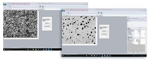
**Ductile Iron**— Nodularity is determined quickly and efficiently with a minimal level of effort and user involvement. Pearlite, Ferrite, and Carbides can also be included in one analysis.
