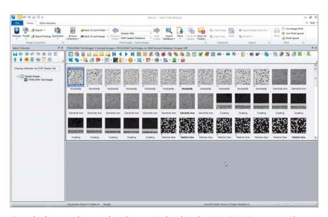
Sample data can be saved and organized within the IA44/PAX-it system with a familiar file cabinet layout. An optional CD creator module is available to save images and data outside your hard drive, while still keeping the IA44/PAX-it format for easy image/data retrieval.
